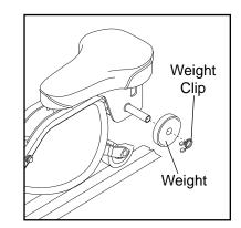
the weights with the weight clips. Note: Place an equal amount of weight on each side of the weight bar. The total combined weight of the user and added weights should not exceed 300 pounds.
